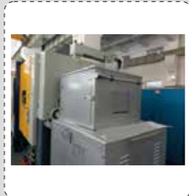
Furnace safety guard
