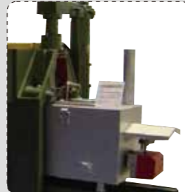
Gas or Diesel heating furnace replace electrical furnace
