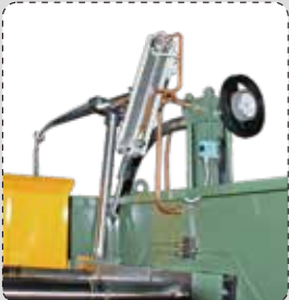
Pneumatic sweeper for casting removal
